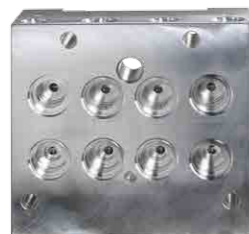
Workpiece: ABS breaking valve Material: Aluminum alloy
