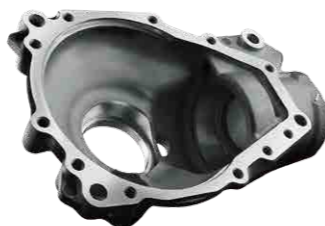
Workpiece: Differential cover Material: Aluminum alloy
